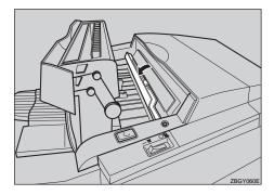
Push the front cover release button and open the front cover.
